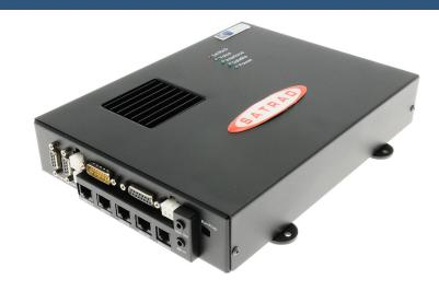
Network Innovations' SATRAD Network Bridge provides autofailover for trunked radio networks to the SATRAD satellite network to ensure uninterrupted remote communications.
