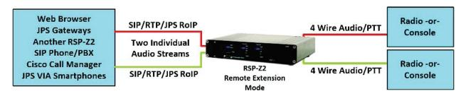
In Cross-Connected Mode, the RSP-Z2 can patch together its two analog ports. If desired, this combined audio can be sent via IP in a single stream, using the desired transport protocol.
